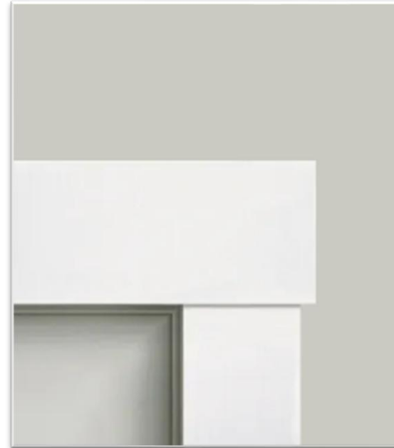
CRAFTSMAN CASING W/ 1x4 LEGS & 1x6 HEADER LEFT "PROUD" EXTENDING 1" PAST 1x4 ON EACH SIDE
